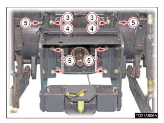
4. Insert the height adjustment hitch bracket ass'y (it assembled in Step 3) to the stud bolt of the transmission case and tighten the spring washers (3), nuts (4) and washer bolts (5).
