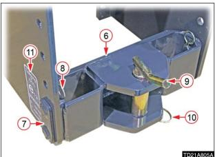
3. After inserting the height adjustment hitch ass'y (6) to the hole of the height adjustment hitch bracket ass'y (1), secure it with the hitch adjustment pin (7), snap pin (8) and attach the hitch certificate label. Install the hitch pin ass'y (9) to the height adjustment hitch bracket and secure it with the clip pin (10).
