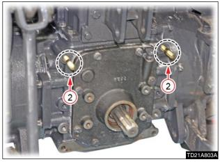
2. Unscrew the original stud bolt (A) and tighten the kit stud bolt (2).
